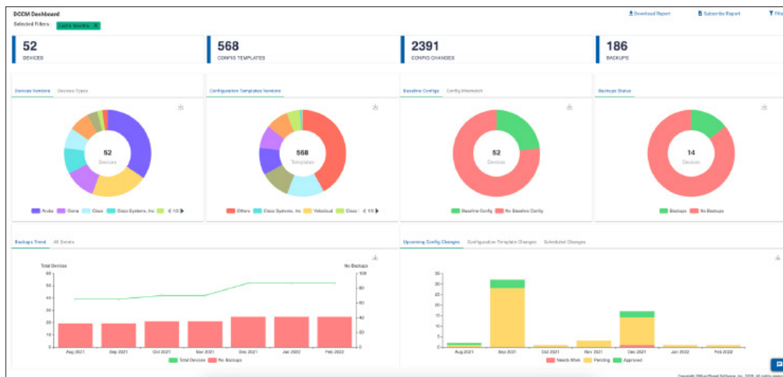
Figure 2. DCCM dashboard enables viewing, analysis, and monitoring of device configuration in real time
